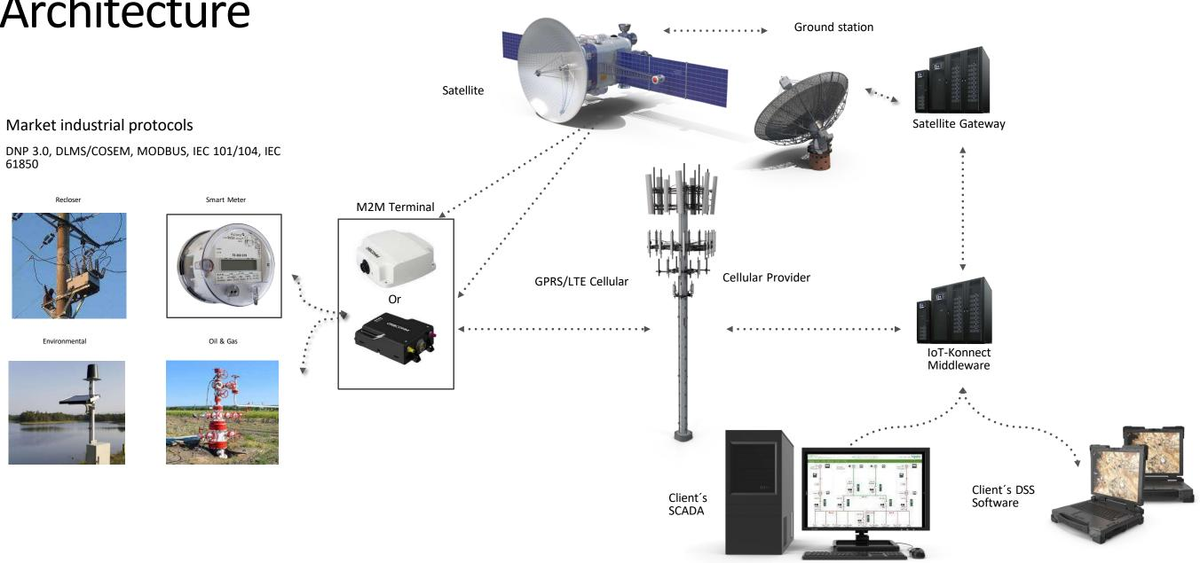
Our M2M terminal installed in the field is fully programmable and is in charge of communicate the slave device with your SCADA or DSS software. The signals are sent through a variety of communications options up to our middleware and then to your SCADA or DSS software, using encrypted and secure channels.
